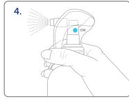
Spray the objects or surfaces both sides from the distance of approx. 20-30 cm with swinging motion.
